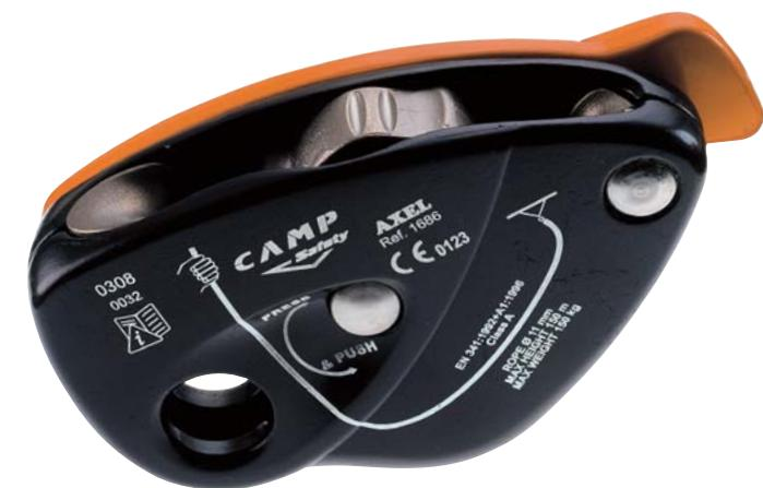
Auto-locking single rope descender and belay device. Can also be used as chest ascender. Two locking positions are engaged by under or over extension of the release handle for maximum safety. Descent speed can be controlled up to 2 m/s. Maximum working load: 150 kg
