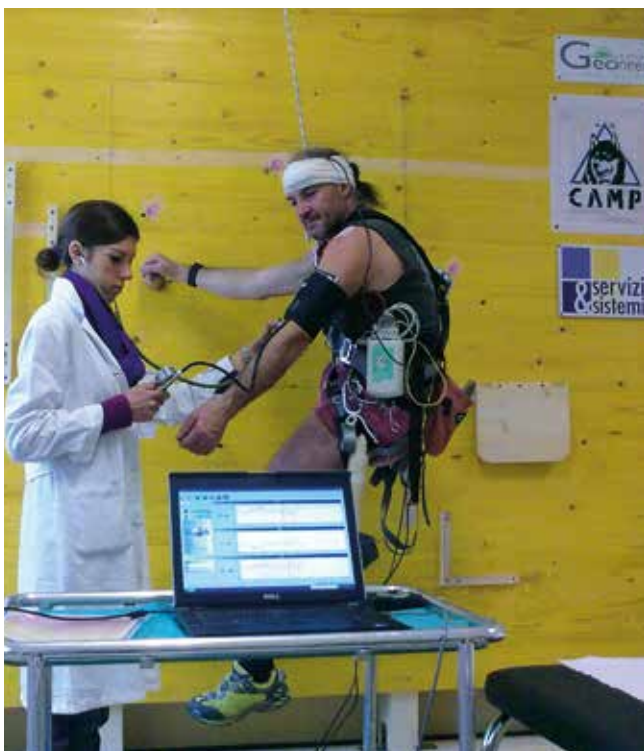
Active and passive suspension test with Golden Top Evo Alu harness. Test de suspensión pasiva y activa con arnés Golden Top Evo Alu. Milano, Italy © Sospesi Project).
