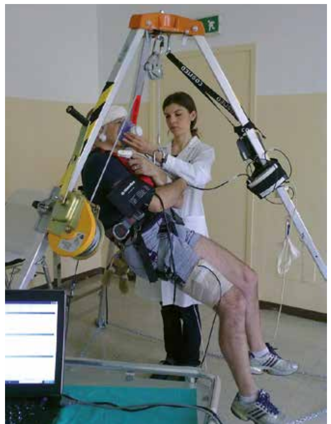
Active and passive suspension test with Golden Top Evo Alu harness. Test de suspensión pasiva y activa con arnés Golden Top Evo Alu. Milano, Italy © Sospesi Project).
